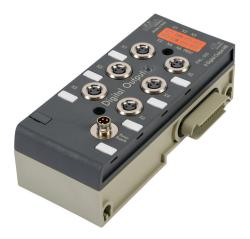
NITRA discrete output module, 6-point, 12-24 VDC, PNP/NPN, 1 common(s), 6 point(s) per common, 1A/point, 4A/common, short circuit and overload protection, IP65. Mounting hardware included. Requires PAL-EIP bus coupler and power cable.
