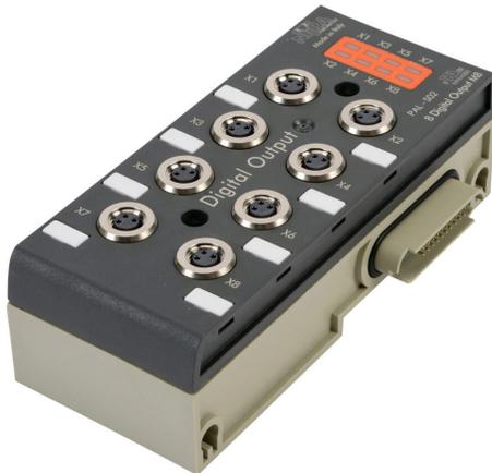
NITRA discrete output module, 8-point, 12-24 VDC, PNP/NPN, 1 common(s), 8 point(s) per common, 1A/point, 4A/common, short circuit and overload protection, IP65. Mounting hardware included. Requires PAL-EIP bus coupler.
