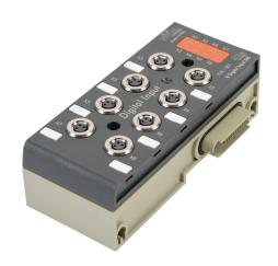
NITRA discrete input module, 8-point, 12-24 VDC, PNP/NPN, 1 common(s), 8 point(s) per common, IP65. For use with PAL series. Mounting hardware included. Requires PAL-EIP bus coupler.
