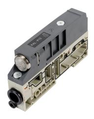
NITRA pneumatic compressed air module, left supply/exhaust, Cv=3.76, 1/2in push-to-connect tubing inlet(s), silenced exhaust(s), 5/32in (4mm) push-to-connect tubing pilot(s), IP65. For use with PAL series.
