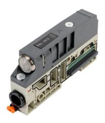
NITRA pneumatic air module, intermediate through, Cv=3.76, 1/2in push-to-connect tubing inlet(s), 5/32in (4mm) push-to-connect tubing pilot(s), IP65. For use with PAL series. Without additional power connection.
