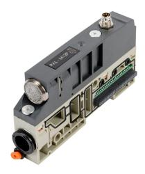
NITRA pneumatic air module, intermediate through, Cv=3.76, 1/2in push-to-connect inlet(s), 5/32in (4mm) push-to-connect pilot(s), IP65. For use with PAL series. Requires power cable. With additional power connection.
