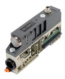
NITRA pneumatic air module, intermediate through, Cv=3.76, 1/2in push-to-connect tubing inlet(s), 5/32in (4mm) push-to-connect tubing pilot(s), IP65. For use with PAL series. Requires power cable. With additional power connection.
