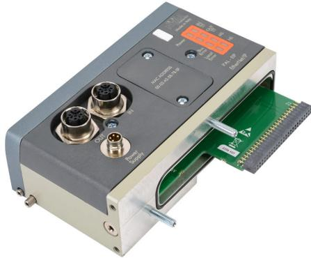
NITRA bus coupler, 12-24 VDC, (2) Ethernet 10/100Base-T (M12) port(s), EtherNet/IP, 10/100 Mbps, (128) solenoid(s) per system, IP65. For use with PAL series. Requires 4-pin M8 power cable.
