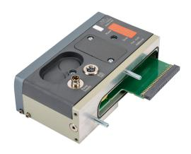
NITRA local expansion coupler, 12-24 VDC, (1) 4-pin M8 quick-disconnect port(s), number of solenoid(s) inclusive of main system, IP65. For use with PAL series. Requires 4-pin M8 power cable.
