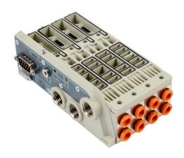
NITRA pneumatic stand-alone valve base, fiberglass-reinforced thermoplastic, (8) solenoid(s), (4) stations, (1) 1/4in female NPT inlet(s), (8) 1/4in push-to-connect outlet(s), (2) 1/4in female NPT exhaust(s), IP65. For use with PAL series.
