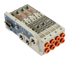
NITRA pneumatic stand-alone valve base, fiberglass-reinforced thermoplastic, (4) solenoid(s), (4) stations, (1) 1/4in female NPT inlet(s), (8) 1/4in push-to-connect outlet(s), (2) 1/4in female NPT exhaust(s), IP65. For use with PAL series.
