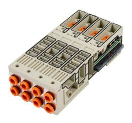
NITRA pneumatic modular valve base, fiberglass-reinforced thermoplastic, (4) solenoid(s), (4) stations, (8) 1/4in push-to-connect tubing outlet(s), IP65. For use with PAL series.
