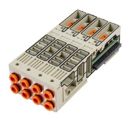
NITRA pneumatic modular valve base, fiberglass-reinforced thermoplastic, (4) solenoid(s), (4) stations, (8) 1/4in push-to-connect outlet(s), IP65. For use with PAL series.
