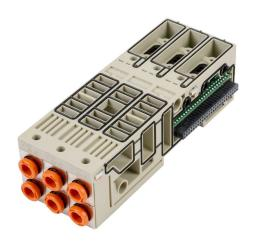
NITRA pneumatic modular valve base, fiberglass-reinforced thermoplastic, (6) solenoid(s), (3) stations, (6) 1/4in push-to-connect outlet(s), IP65. For use with PAL series.
