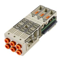
NITRA pneumatic modular valve base, fiberglass-reinforced thermoplastic, (3) solenoid(s), (3) stations, (6) 1/4in push-to-connect tubing outlet(s), IP65. For use with PAL series.
