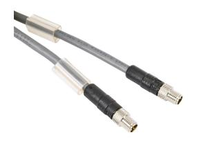
NITRA expansion cable, 4-pin M8 axial male to 4-pin M8 axial male, IP65, 16.4ft/5m cable length. For use with PAL series bus expansion coupler.
