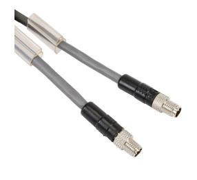
NITRA expansion cable, 4-pin M8 axial male to 4-pin M8 axial male, IP65, 3.2ft/1m cable length. For use with PAL series bus expansion coupler.
