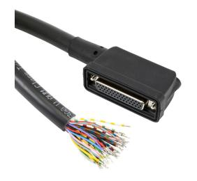
NITRA control cable, 44-pin D-sub right-angle female to pigtail, IP65, 8.2ft/2.5m cable length. For use with PAL-E44 electrical connection module.
