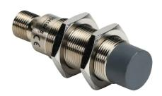
AchieVe inductive proximity sensor, tubular, 18mm diameter x 63.5mm body, nickel-plated brass housing, PNP, N.O. output, 8mm sensing distance, non-flush, 2 kHz switching frequency, IP67, 4-pin M12 quick-disconnect.
