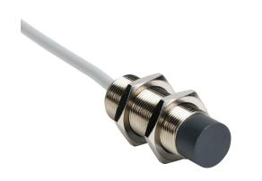
AchieVe inductive proximity sensor, tubular, 18mm diameter x 50mm body, nickel-plated brass housing, PNP, N.O. output, 8mm sensing distance, non-flush, 2 kHz switching frequency, IP67, pigtail.
