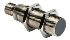
AchieVe inductive proximity sensor, tubular, 18mm diameter x 63.5mm body, nickel-plated brass housing, PNP, N.O. output, 5mm sensing distance, flush, 2 kHz switching frequency, IP67, 4-pin M12 quick-disconnect.
