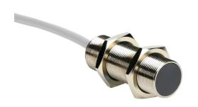
AchieVe inductive proximity sensor, tubular, 18mm diameter x 50mm body, nickel-plated brass housing, PNP, N.O. output, 5mm sensing distance, flush, 2 kHz switching frequency, IP67, pigtail.
