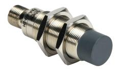
AchieVe inductive proximity sensor, tubular, 18mm diameter x 63.5mm body, nickel-plated brass housing, NPN, N.O. output, 8mm sensing distance, non-flush, 2 kHz switching frequency, IP67, 4-pin M12 quick-disconnect.
