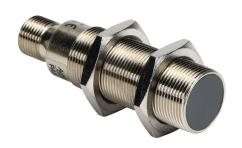
AchieVe inductive proximity sensor, tubular, 18mm diameter x 63.5mm body, nickel-plated brass housing, NPN, N.O. output, 5mm sensing distance, flush, 2 kHz switching frequency, IP67, 4-pin M12 quick-disconnect.
