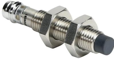
AchieVe inductive proximity sensor, tubular, 8mm diameter x 45mm body, 304 stainless steel housing, PNP, N.O. output, 2.5mm sensing distance, non-flush, 4.5 kHz switching frequency, IP67, 3-pin M8 quick-disconnect.
