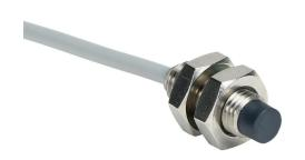
AchieVe inductive proximity sensor, tubular, 8mm diameter x 22mm body, 304 stainless steel housing, PNP, N.O. output, 2.5mm sensing distance, non-flush, 4.5 kHz switching frequency, IP67, pigtail.
