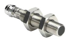
AchieVe inductive proximity sensor, tubular, 8mm diameter x 45mm body, 304 stainless steel housing, PNP, N.O. output, 1.5mm sensing distance, flush, 5 kHz switching frequency, IP67, 3-pin M8 quick-disconnect.
