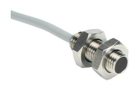
AchieVe inductive proximity sensor, tubular, 8mm diameter x 22mm body, 304 stainless steel housing, PNP, N.O. output, 1.5mm sensing distance, flush, 5 kHz switching frequency, IP67, pigtail.
