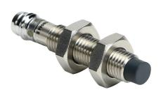
AchieVe inductive proximity sensor, tubular, 8mm diameter x 45mm body, 304 stainless steel housing, NPN, N.O. output, 2.5mm sensing distance, non-flush, 4.5 kHz switching frequency, IP67, 3-pin M8 quick-disconnect.
