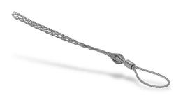
Bryant light-duty pulling grip, low tension, accepts cable diameter size 1.25 to 1.49in, closed single weave, galvanized steel mesh, 14in length, flexible, eye length 7in.
