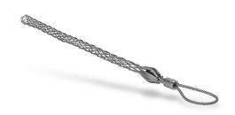
Bryant light-duty pulling grip, low tension, accepts cable diameter size 0.75 to 0.99in, closed single weave, galvanized steel mesh, 12in length, flexible, eye length 6in.
