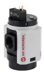
Norgren soft start valve, 3-port (3-way), 2-position, single solenoid spring return, N.C., 3/4in female NPT inlet(s), 3/4in female NPT outlet(s), 1/2in female NPT exhaust(s), Cv=4, 24 VDC operating voltage. For use with Excelon Plus 84 series components.
