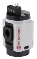
Norgren soft start valve, 3-port (3-way), 2-position, single solenoid spring return, N.C., 1/2in female NPT inlet(s), 1/2in female NPT outlet(s), 1/2in female NPT exhaust(s), Cv=4, 24 VDC operating voltage. For use with Excelon Plus 84 series components.
