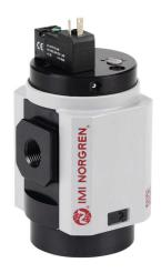
Norgren soft start valve, 3-port (3-way), 2-position, single solenoid spring return, N.C., 3/8in female NPT inlet(s), 3/8in female NPT outlet(s), 1/2in female NPT exhaust(s), Cv=2.9, 24 VDC operating voltage. For use with Excelon Plus 84 series components.
