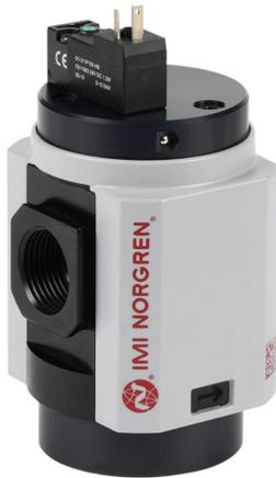
Norgren shut-off valve, 3-port (3-way), 2-position, single solenoid spring return, N.C., 3/4in female NPT inlet(s), 3/4in female NPT outlet(s), 1/2in female NPT exhaust(s), Cv=4.6, 24 VDC operating voltage. For use with Excelon Plus 84 series components.
