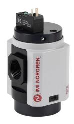
Norgren shut-off valve, 3-port (3-way), 2-position, single solenoid spring return, N.C., 3/4in female NPT inlet(s), 3/4in female NPT outlet(s), 1/2in female NPT exhaust(s), Cv=4.6, 24 VDC operating voltage. For use with Excelon Plus 84 series components.
