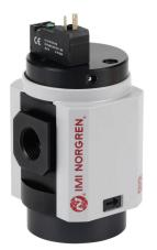
Norgren shut-off valve, 3-port (3-way), 2-position, single solenoid spring return, N.C., 1/2in female NPT inlet(s), 1/2in female NPT outlet(s), 1/2in female NPT exhaust(s), Cv=4.6, 24 VDC operating voltage. For use with Excelon Plus 84 series components.
