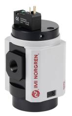
Norgren shut-off valve, 3-port (3-way), 2-position, single solenoid spring return, N.C., 3/8in female NPT inlet(s), 3/8in female NPT outlet(s), 1/2in female NPT exhaust(s), Cv=3, 24 VDC operating voltage. For use with Excelon Plus 84 series components.
