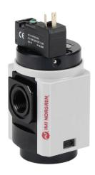
Norgren soft start valve, 3-port (3-way), 2-position, single solenoid spring return, N.C., 3/8in female NPT inlet(s), 3/8in female NPT outlet(s), 1/4in female NPT exhaust(s), Cv=1.8, 24 VDC operating voltage. For use with Excelon Plus 82 series components.
