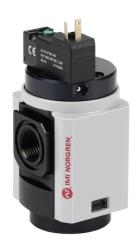
Norgren shut-off valve, 3-port (3-way), 2-position, single solenoid spring return, N.C., 3/8in female NPT inlet(s), 3/8in female NPT outlet(s), 1/4in female NPT exhaust(s), Cv=1.8, 24 VDC operating voltage. For use with Excelon Plus 82 series components.
