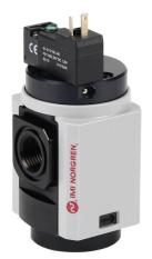
Norgren shut-off valve, 3-port (3-way), 2-position, single solenoid spring return, N.C., 3/8in female NPT inlet(s), 3/8in female NPT outlet(s), 1/4in female NPT exhaust(s), Cv=1.8, 24 VDC operating voltage. For use with Excelon Plus 82 series components.
