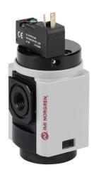
Norgren shut-off valve, 3-port (3-way), 2-position, single solenoid spring return, N.C., 1/4in female NPT inlet(s), 1/4in female NPT outlet(s), 1/4in female NPT exhaust(s), Cv=1.6, 24 VDC operating voltage. For use with Excelon Plus 82 series components.
