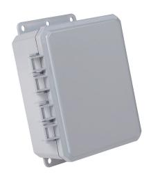
Integra Impact series enclosure, NEMA 1/2/3/3R/3S/4/4X/6/6P/12/13, 8 x 6 x 3in (HxWxD), wall mount, polycarbonate, gray, gloss finish, single-door, integrated padlockable latch.
