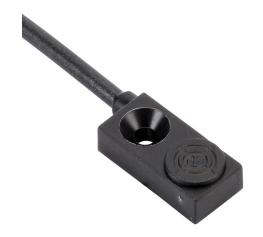
ProSense inductive proximity sensor, rectangular, 8 x 4.7 x 16mm body, polyamide housing, top sensing, PNP, N.C. output, 2.5mm sensing distance, non-flush, 3 kHz switching frequency, IP67, 3-pin M8 quick-disconnect.
