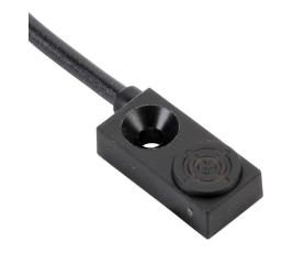
ProSense inductive proximity sensor, rectangular, 8 x 4.7 x 16mm body, polyamide housing, top sensing, PNP, N.C. output, 1.5mm sensing distance, flush, 2.5 kHz switching frequency, IP67, 3-pin M8 quick-disconnect.
