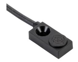
ProSense inductive proximity sensor, rectangular, 8 x 4.7 x 16mm body, polyamide housing, top sensing, PNP, N.O. output, 2.5mm sensing distance, non-flush, 3 kHz switching frequency, IP67, 3-pin M8 quick-disconnect.
