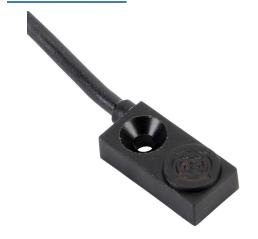
ProSense inductive proximity sensor, rectangular, 8 x 4.7 x 16mm body, polyamide housing, top sensing, PNP, N.O. output, 1.5mm sensing distance, flush, 2.5 kHz switching frequency, IP67, 3-pin M8 quick-disconnect.
