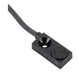
ProSense inductive proximity sensor, rectangular, 8 x 4.7 x 16mm body, polyamide housing, top sensing, NPN, N.O. output, 2.5mm sensing distance, non-flush, 2.5 kHz switching frequency, IP67, pigtail.
