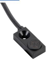
ProSense inductive proximity sensor, rectangular, 8 x 4.7 x 16mm body, polyamide housing, top sensing, NPN, N.O. output, 1.5mm sensing distance, flush, 2.5 kHz switching frequency, IP67, 3-pin M8 quick-disconnect.
