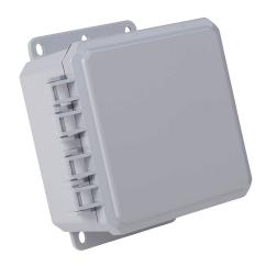
Integra Impact series enclosure, NEMA 1/2/3/3R/3S/4/4X/6/6P/12/13, 6 x 6 x 3in (HxWxD), wall mount, polycarbonate, gray, gloss finish, single-door, integrated padlockable latch.
