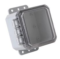
Integra Impact series enclosure, NEMA 1/2/3/3R/3S/4/4X/6/6P/12/13, 4 x 4 x 3in (HxWxD), wall mount, polycarbonate, gray, gloss finish, clear polycarbonate single-door, integrated padlockable latch.
