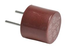
Productivity3000 spare fuse, 3.15A. Package of 5. For use with P3-08TAS and P3-08TRS output modules.
