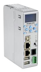
Productivity3000 CPU, up to 50 MB ladder memory, 4 x 10 character LCD display, USB A storage, (2) Ethernet 10/100Base-T (RJ45), (1) RS-232/RS-485 (RJ12), (1) RS-232/RS-485 (4-pin terminal), (1) USB A expansion and (1) USB B port(s), battery included.
