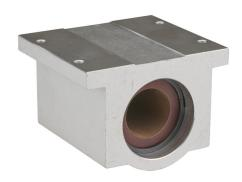
PBC Simplicity series single pillow block, plain bearing, 3.63in overall length, PTFE, 1-1/4in inside diameter, aluminum housing, 0.0005in running clearance. For use with 1-1/4in diameter PBC shafts.
